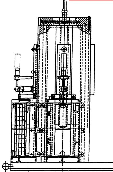
Figure 7 Fast CTE Test Set
