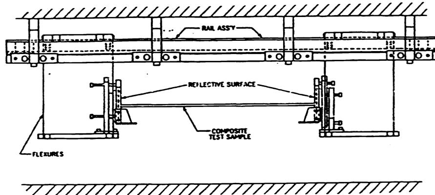
Figure 2 Coupon Support Assembly
